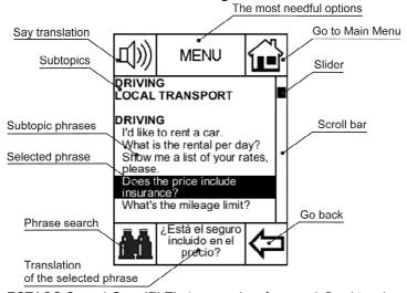
ECTACO SpeechGuard™ TL-4 screen has four predefined touchsensitive areas located in the corners of the display. Depending on the section, these areas hold the following touch buttons.
